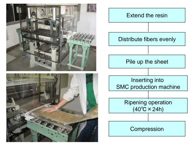
Fig.1 New small SMC production machine
